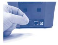
STEP 7 - Load the printer driver from the CD or a web download file and set up the ethernet port and IP address.
